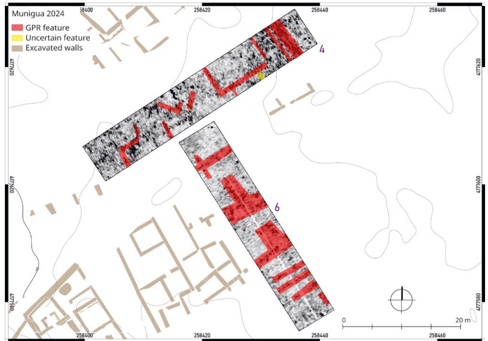
Fig. 4: Area 2a with single timeslices around 0.4 m depth (top) and highlighted features in the grayscale image (bottom). (Grid 4: 7.7317 ns, 0.38659 m; Grid 6: 7.4285 ns, 0.37143 m).
