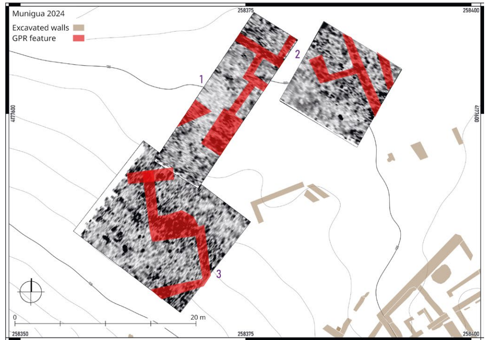
Fig. 3: Area 1 with single timeslices around 0.4 m depth (top) and highlighted features in the grayscale image (bottom). (Grid 1: 8.0349 ns, 0.40175 m; Grid 2: 7.4285 ns, 0.37143 m; Grid 3: 7.8833 ns, 0.39417 m.).
