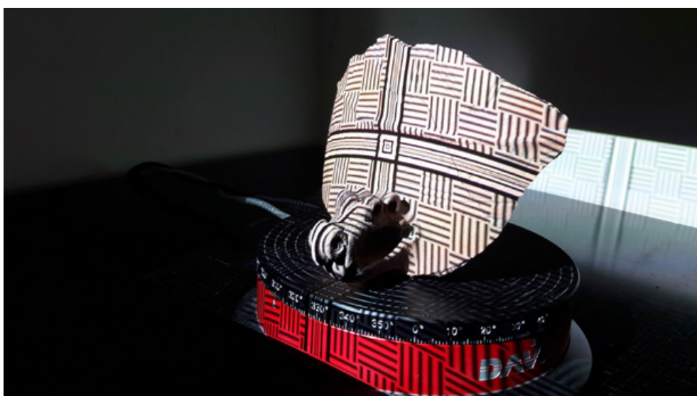
Fig. 15: Sherd on the turntable with structured-light pattern
