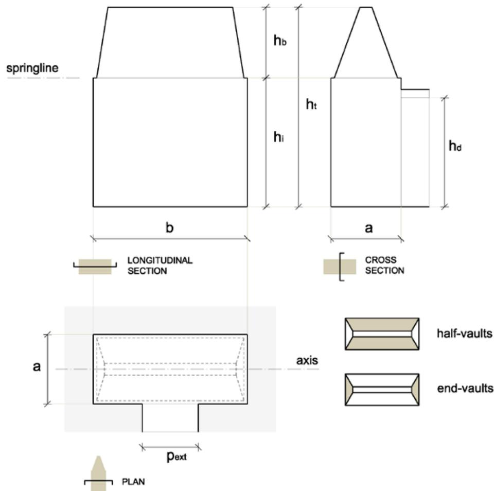
Fig. 12: Vaults geometrical variables
