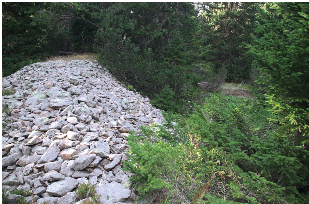
Fig. 6: Stone clearance dumps from washing operations within the opencast at Crvene Zemlje
