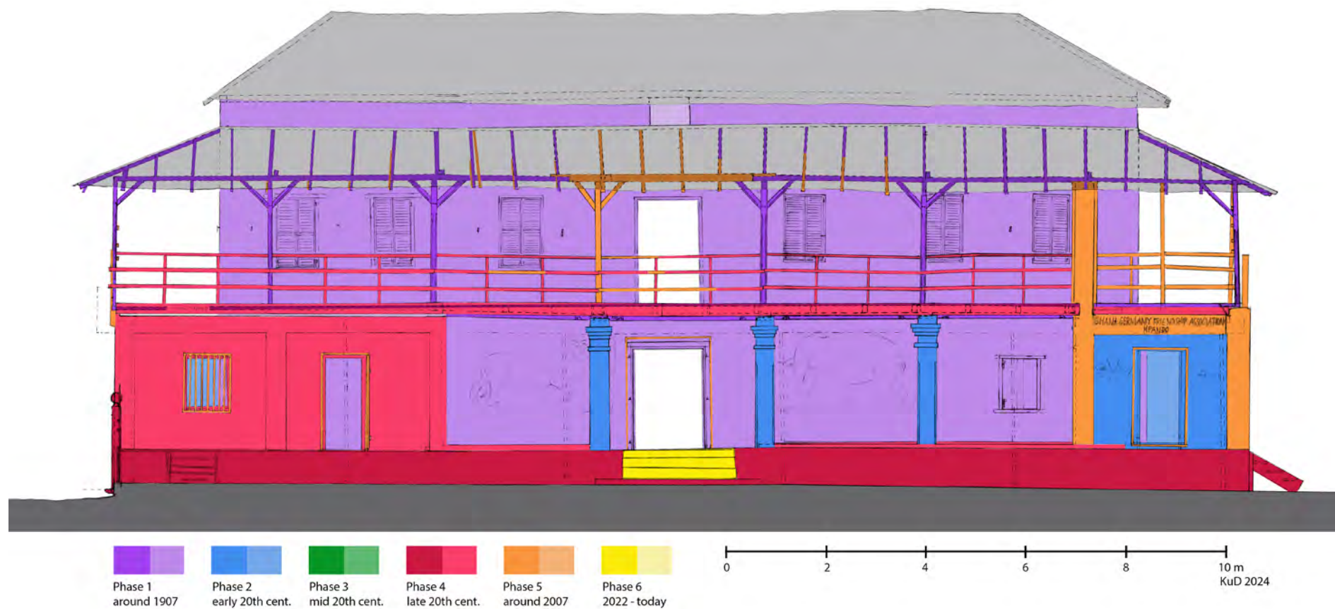
Fig. 4: Kpando, Ghana. Plan of building phases of the south elevation of the main building of the palace compound
