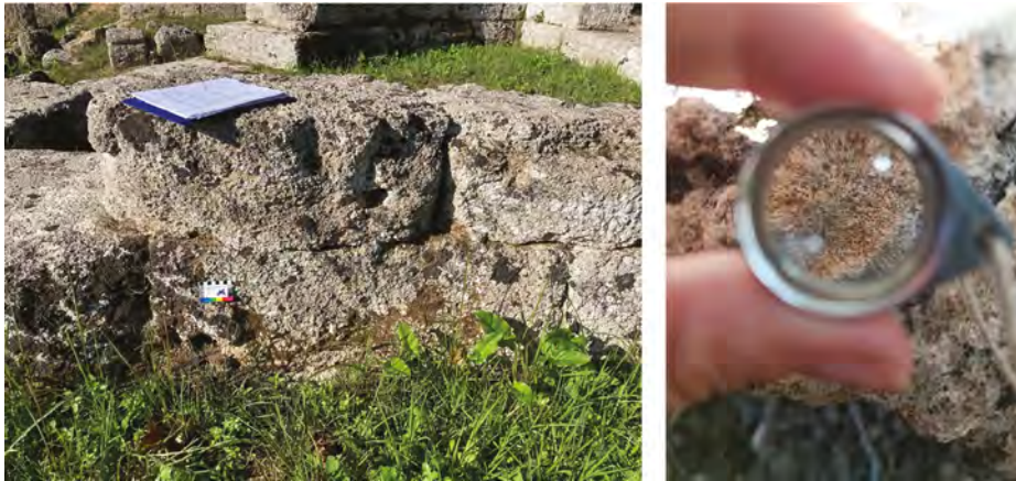
Fig. 1: Equipment for macroscopic geological study of the building stone. Left: photo of the site, with scale and printed map of the stones of the building being studied (Buleuterion) for compiling data. Right: view through a mineralogist's magnifying glass (up to x10), classic equipment for description in fieldwork
