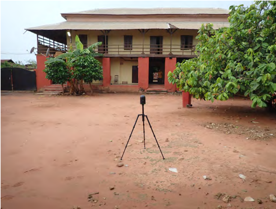
Fig. 2: Kpando, Ghana. Digital 3D documentation. Imaging Laser Scanner Leica BLK in operation in the courtyard of the Palace of the Paramount Chief with a view to its northern façade
