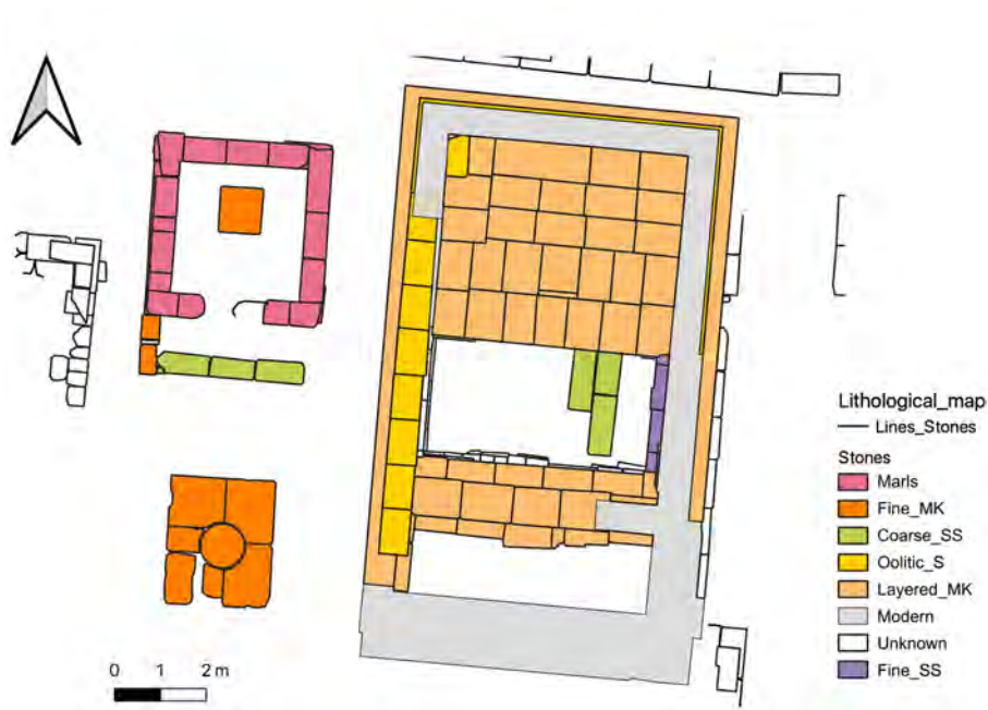
Fig. 3: Lithological map of Foundations B, C and 1 in the Altis treasuries at Olympia showing different facies and the variability of the shelly facies, which exhibit different characteristics. On QGIS, ongoing work with provisional names (MK=Muschelkalk; SS=Sandstone; S=Stone)
