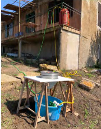
Fig. 20: Simplified flotation system with water recycling
