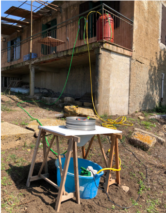
Fig. 20: Simplified flotation system with water recycling
