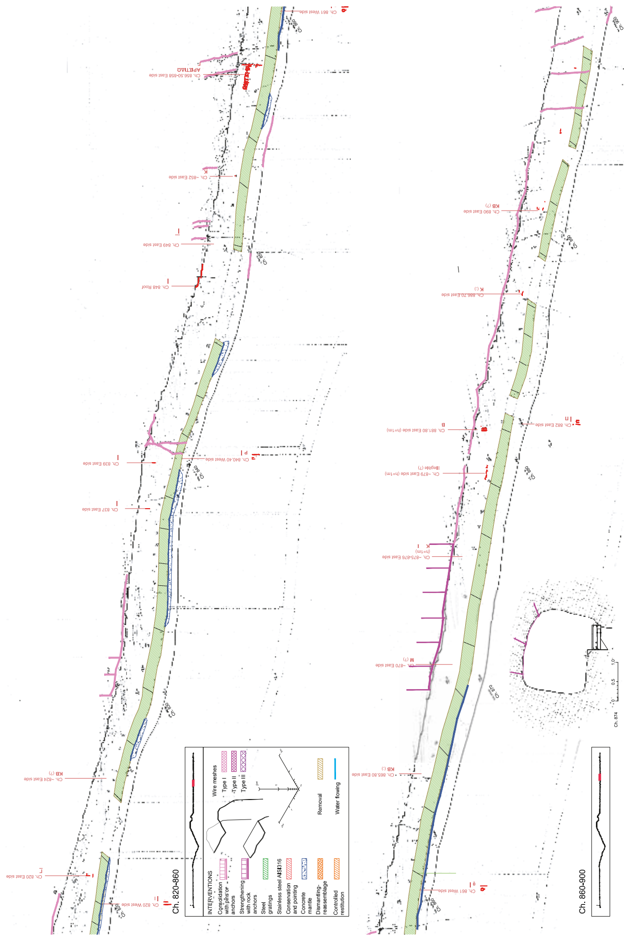
Fig. 15. Isometric plan of the tunnel of Eupalinos (scale 1 : 200) with sections (scale 1 : 100), Ch. 820–860
