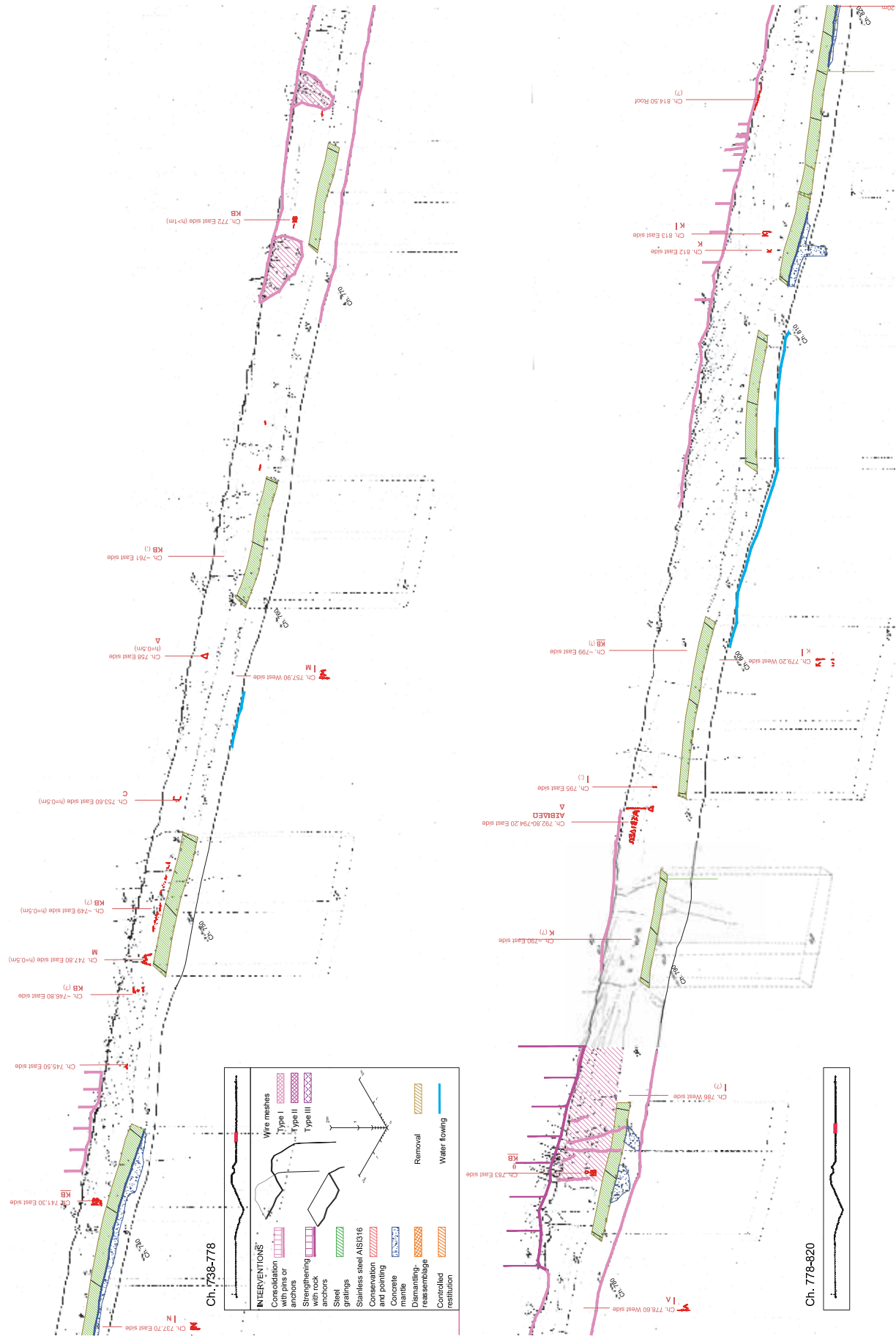
Fig. 14. Isometric plan of the tunnel of Eupalinos (scale 1 : 200) with sections (scale 1 : 100), Ch. 738-820
