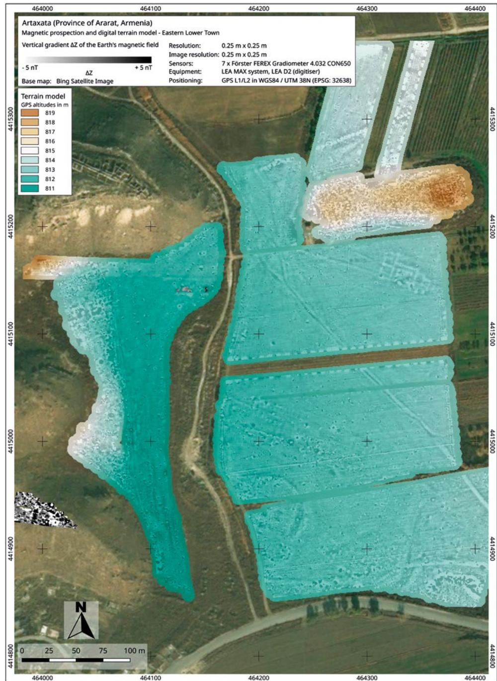
Fig. 8: Artaxata, superimposition of magnetic data and terrain model
