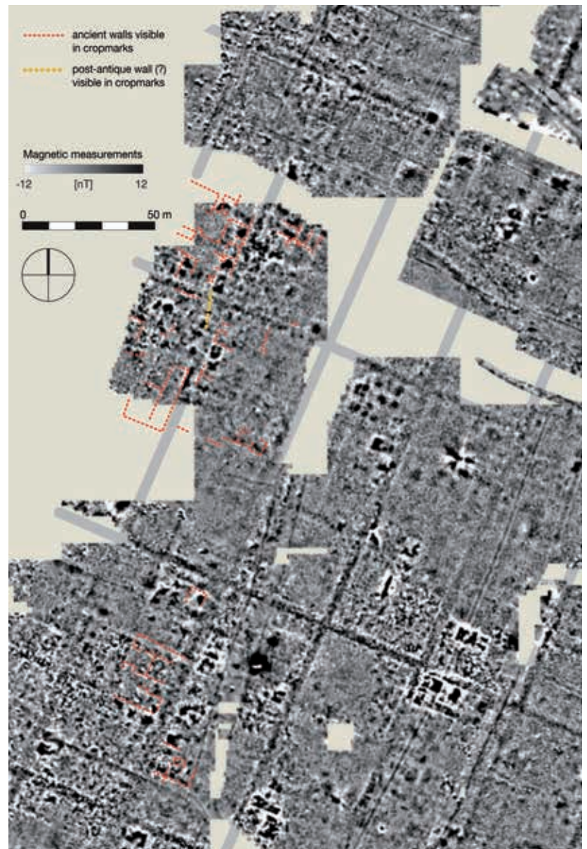
Fig. 5 Miletus, geomagnetic chart of the meadow with cropmarks in the centre of the southern city, opposite the museum (cf. Fig. 2); most cropmarks (red) correspond with buildings on the ancient insulae that show up as white anomalies in the geomagnetic chart. In contrast, one cropmark (yellow) has a different orientation, overbuilds an ancient street, and does not correspond with any geomagnetic anomaly; this cropmark is probably indicative of a later, Turkish wall (scale 1 : 2000)
