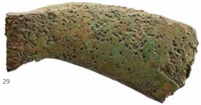
Fig. 29: Gas or blow-holes on the surface of a single-edged shaft-hole broken axe (Cat. 3)
