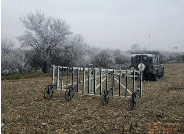
Fig. 3. The vehicle-towed 16-channel magnetometer system (SENSYS MAGNETO®-MX ARCH) at Tolna-Mözs.
