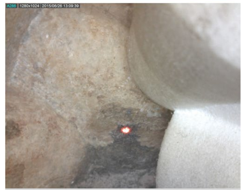
14 Probable effects of 'light and shade' on the north frieze (Gigantomachy), chariot of Themis: shading with a touch of black(?); the red rectangle outlines the area in which a single XRF spectrum was obtained as initially marked by the laser spot in the high resolution photograph. The XRF spectrum clearly reveals the presence of copper (Cu) and zinc (Zn), the main components of brass, in addition other elements.
