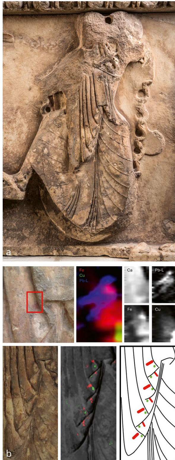
11 Detail of the south frieze showing Athena re-mounting her chariot: a) MA-XRF scan of detail of the himation, illustrating that, next to the visible red paint, traces of lead (Pb) and copper (Cu) based pigments can also be detected. The red shape indicates the investigated area; b) Partial reconstruction of the red and green pattern of Athena’s himation border by means of hyperspectral imaging (west frieze)
