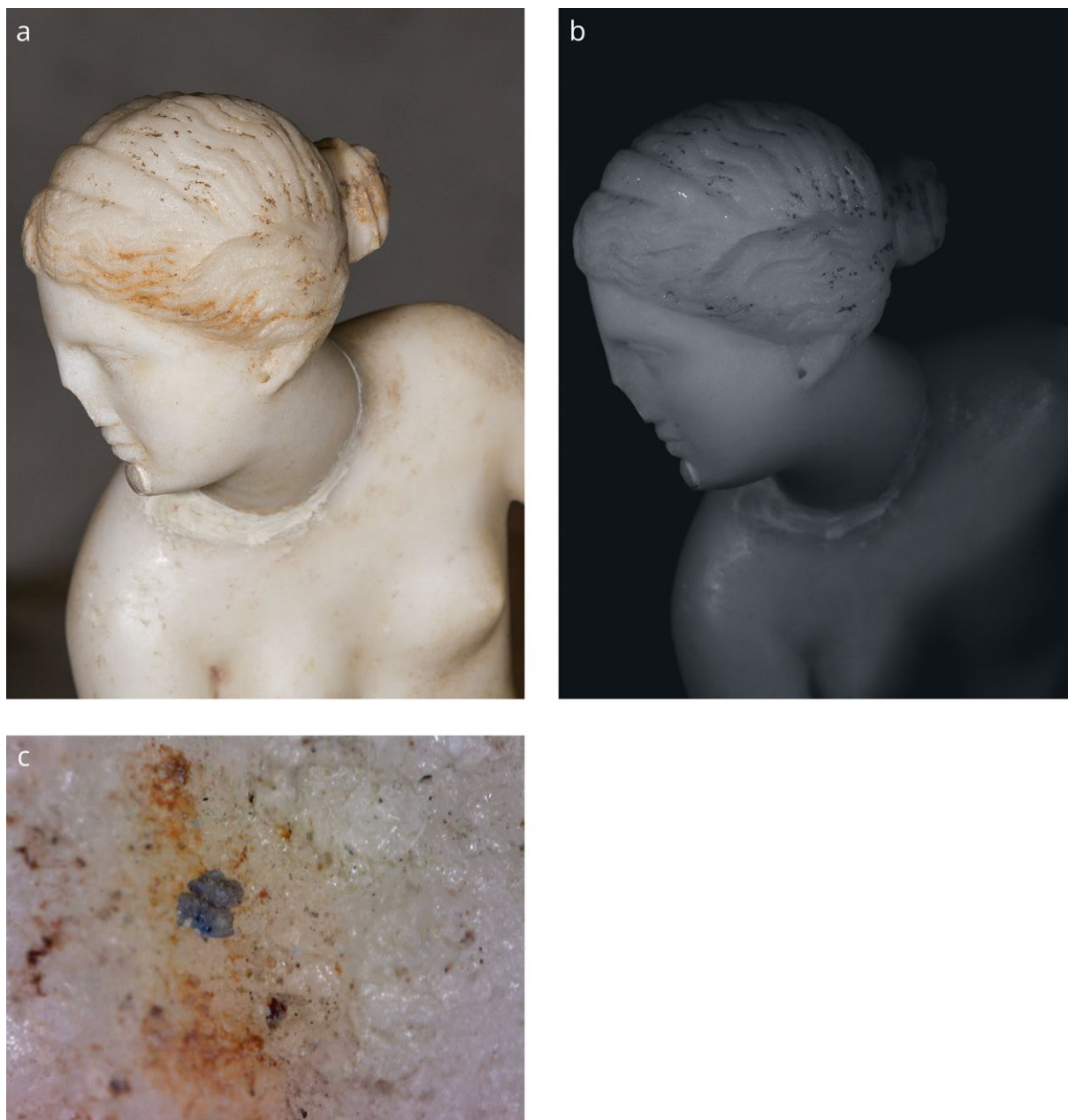
6 a) Detail of Venus's hair; b) VIL images; c) high magnification image of a blue grain
