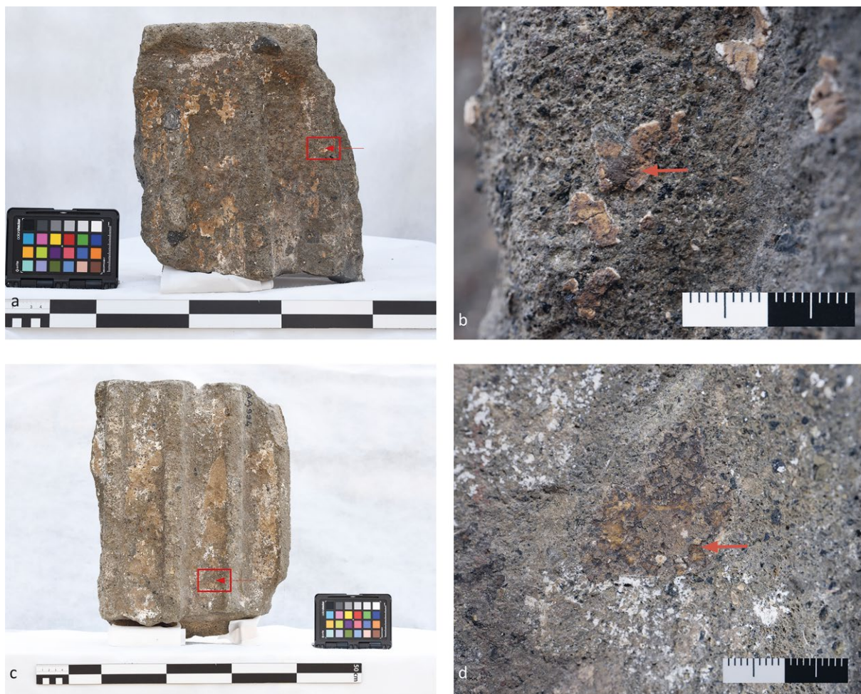
10 Largo Argentina, Temple A, construction phase 1 (c. 240 B.C.). Fragments of column shafts in Lapis Albanus. a. b) Columnar neck fragment (AA 1623) with remains of stucco surface, probably with fire damage, and macrophotography of a detail with location of sample (arrow); c. d) Fragment from the middle of a column shaft (AA 994) and macrophotography of the surface with location of sample (arrow)
