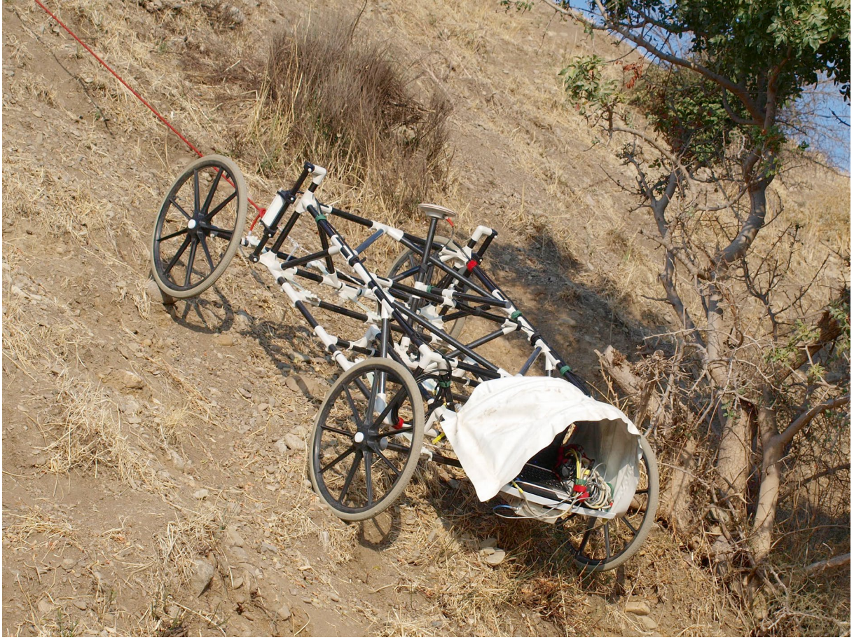
8 Yiğma Tepe, instrument carrier for magnetic sensors lowered on a rope (Photo: W. Rabel)
