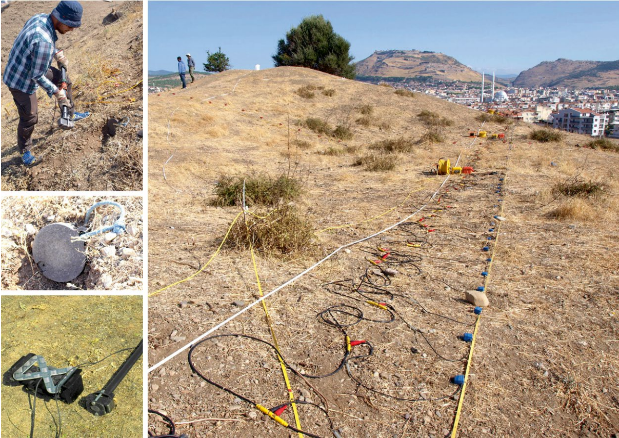
5 Equipment for shear wave measurements: transmission of horizontal forces to the ground (left) and seismic recording line with 0.5 m spaced horizontal geophones (right)
