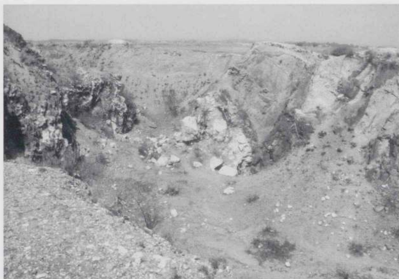
Fig. 20 A large conical hill North of the Weki Duba–Asmara Road, and just North of the Hara Hot gold processing plant. It now appears as a crater, with shafts following veins at the bottom. This is the Gradino or No. 3 mine designated by Usoni (1952).
