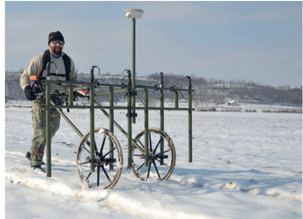
Fig. 4. The 5-channel magnetometer (SENSYS MAGNETO®-MX ARCH) in use (with Gábor Serlegi) at Alsónyék. Sensors spaced at 50 cm intervals.
